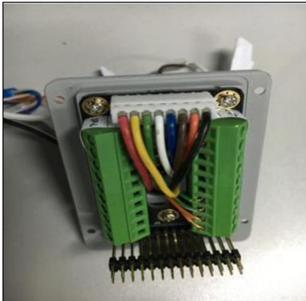
Figure 59: Wiegand Interface Cable
