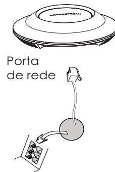
Cabo ethernet RJ45 para o switch PoE (Power over Ethernet)
