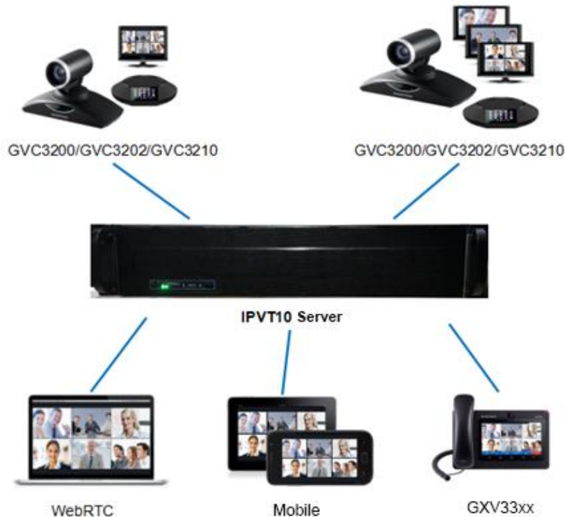
Figure 1: IPVT10 Video Conferencing System Architecture
